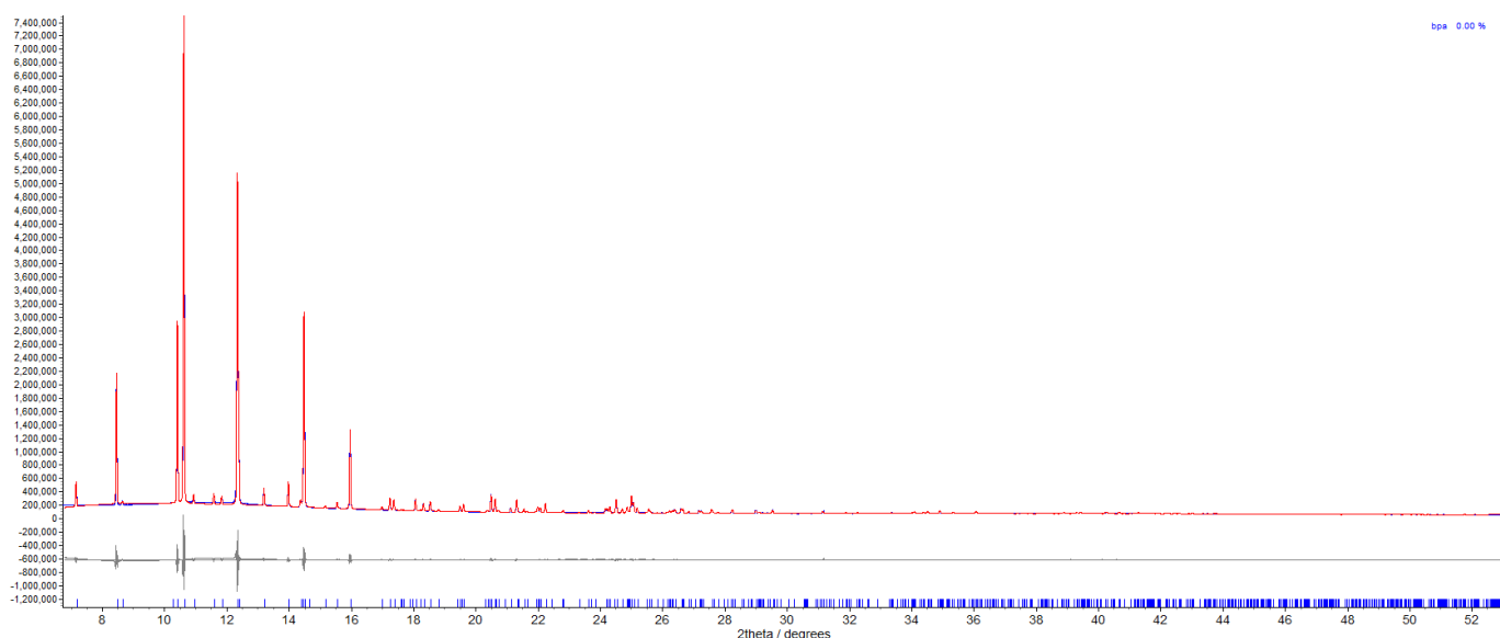
Figure S8.1. Observed (blue) and calculated (red) profiles and difference plot [ I_{obs} - I_{calc} ] (grey) of the Pawley refinement. ( 2\theta range 6.8 - 53^\circ , d_{min} = 0.92 \text{ \AA} ).
