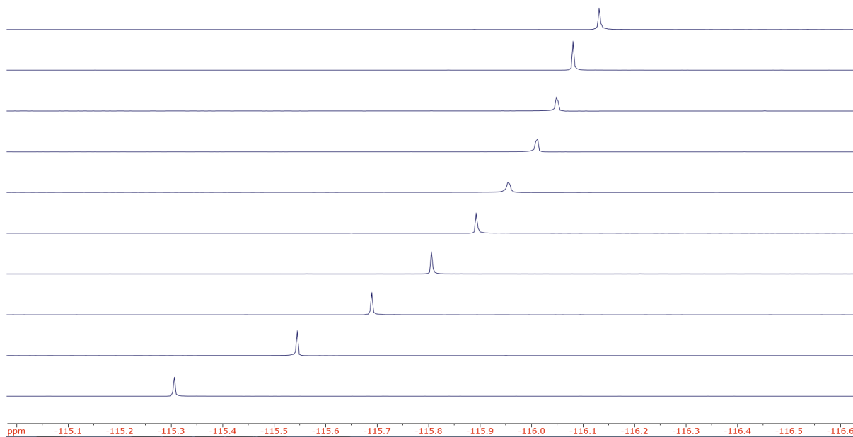
Figure S4.11: partial 376.5 MHz ^{19}\text{F} NMR spectra of titration in chloroform
