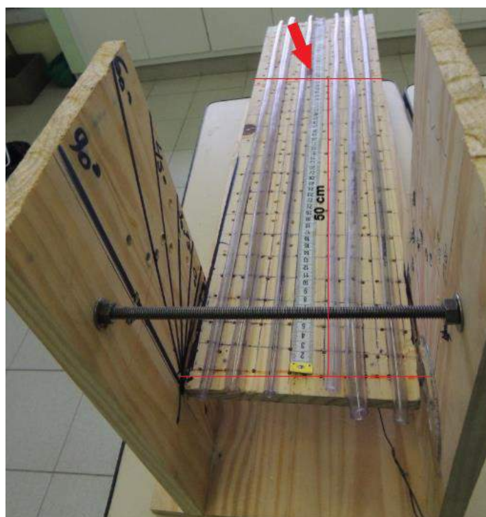
Figure 1. Experimental set up. A silicone tube (50 cm) coupled to an apparatus consisting of a wooden plate (angle 0^\circ ).
