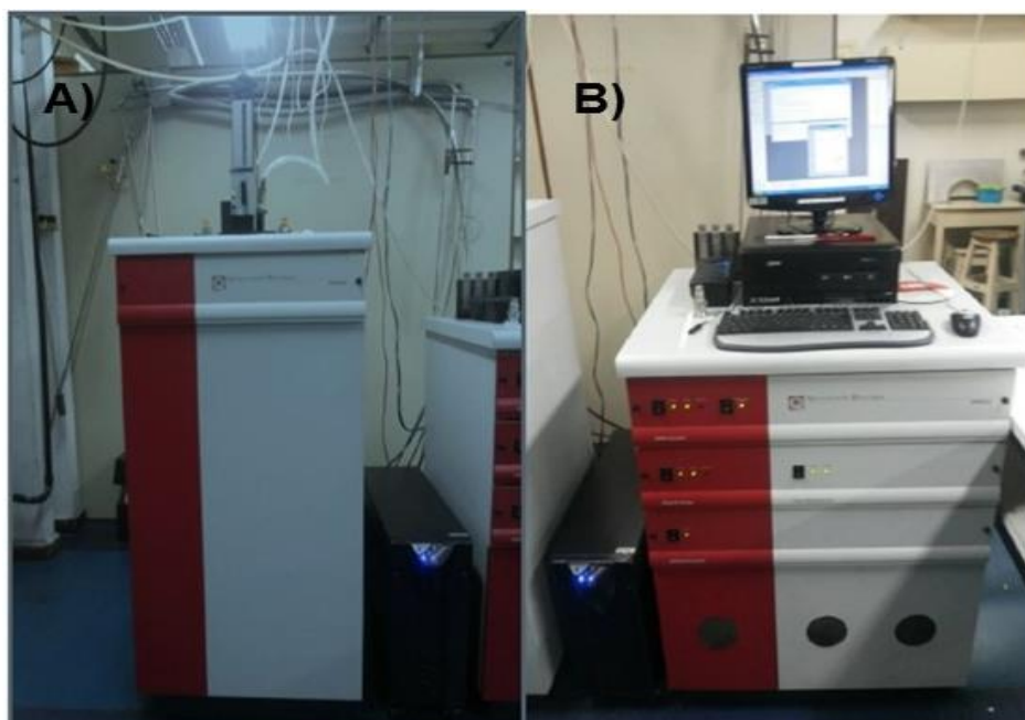
Figura 4.6 - (A-B) Magnetômetro SQUID (“Superconductor Quantum Interference Device”), LSM da UFRGS [73].
