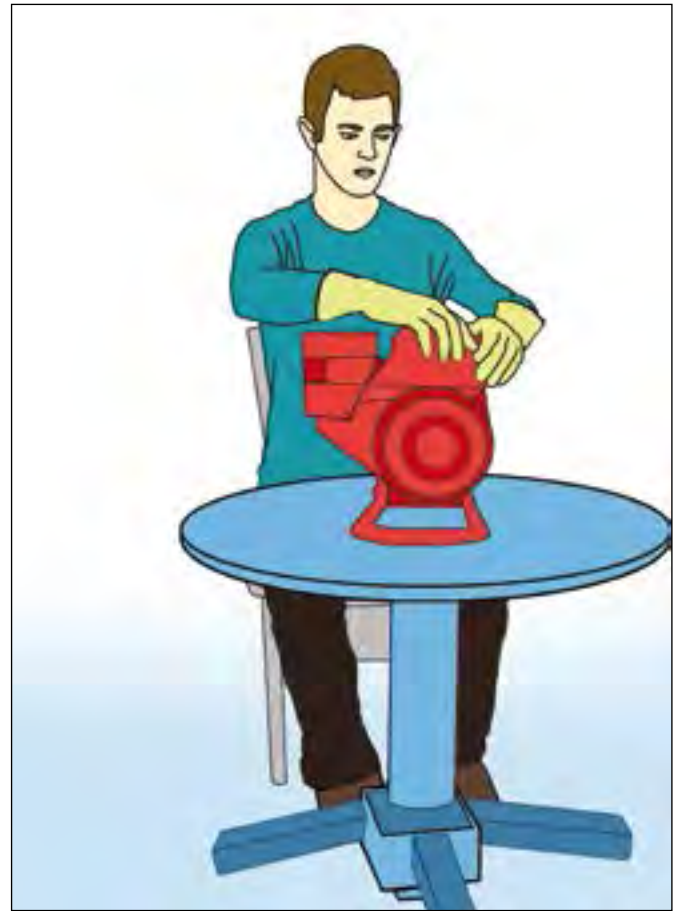
Figure 27b. A rotating stand makes it easy to work on an item from different directions.
