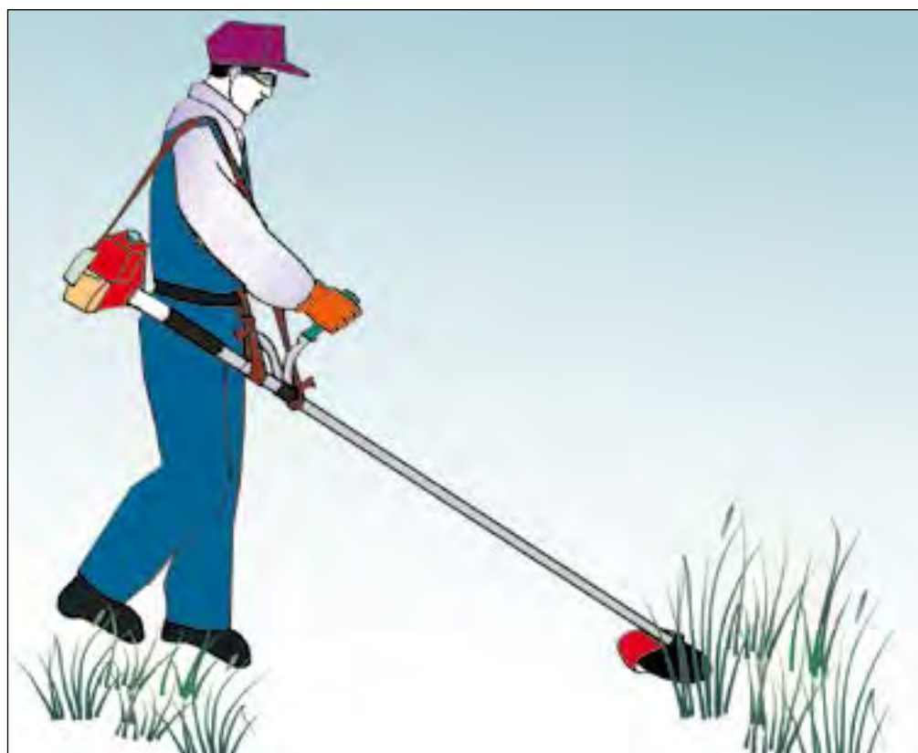
Figure 36b. Hand-held powered tools reduce farmers' workloads. Stable handgrips are essential for safe, productive operation.
