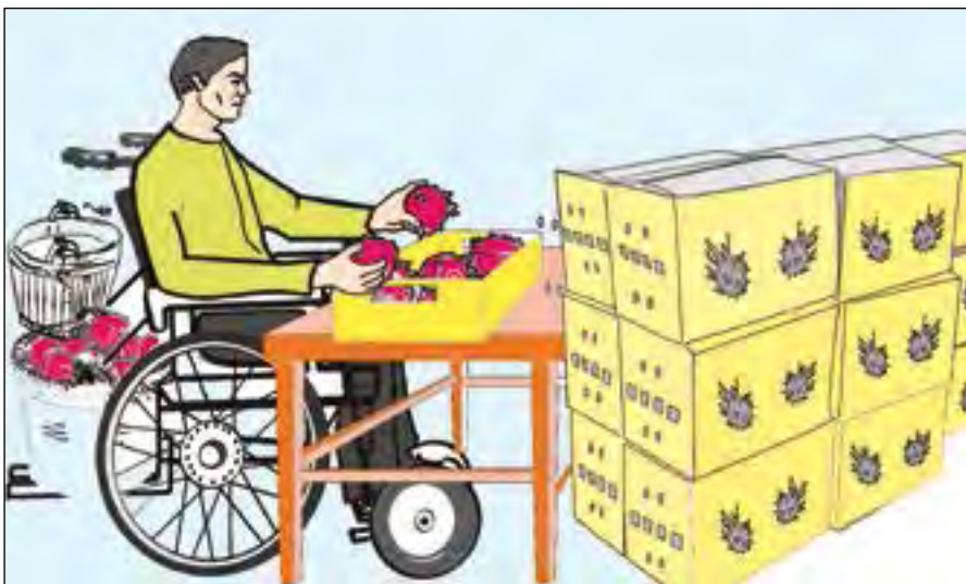
Figure 87b. Provide workstations suited for workers in wheelchairs and other workers with disabilities, so that they can work smoothly and comfortably.
