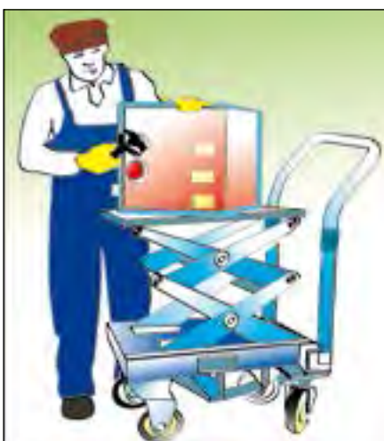
Figure 11d. A manually powered device for lifting heavy items to working level.
