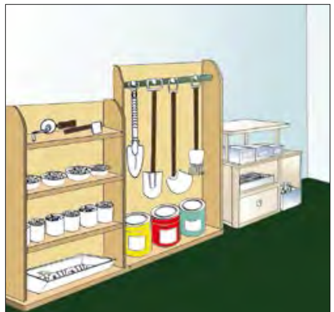
Figure 16d. Multi-level racks to hold agricultural tools. Store small tools or work items in special bins or trays with clear labels.
