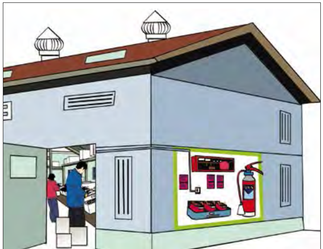
Figure 58. Make sure that appropriate types of fire extinguisher are placed near a work area where there is a risk of fire.
