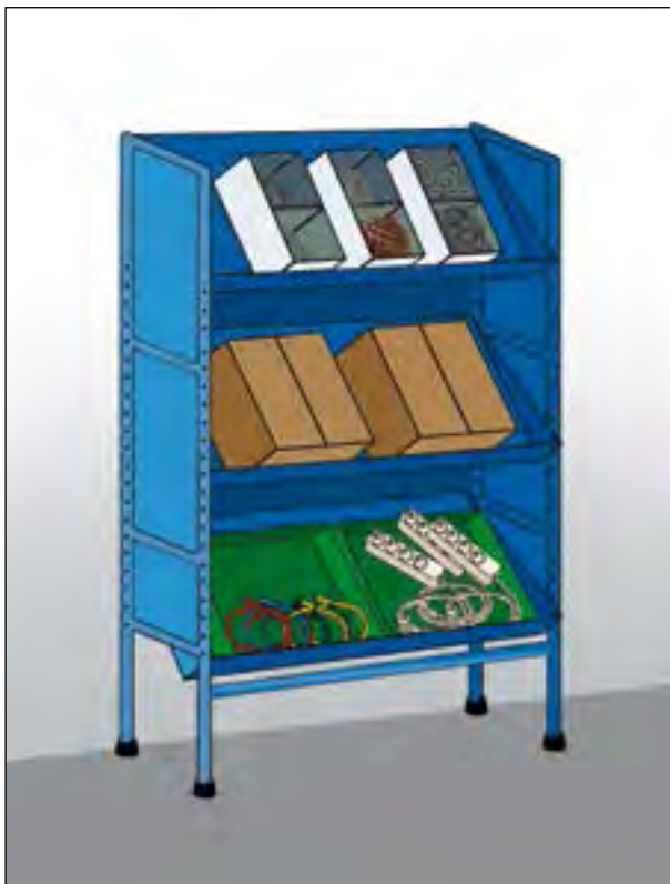
Figure 8d. Multi-level shelves are useful for storing different containers and trays together.
