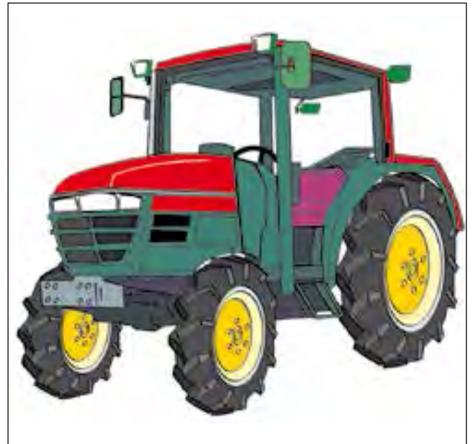
Figure 48b. Mirrors can increase the front and rear views for the driver.
