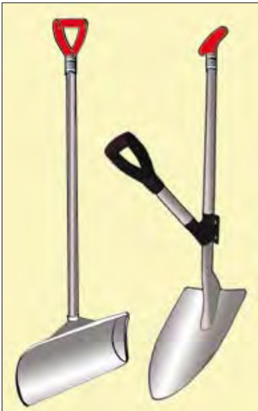
Figure 25d. The handles of tools should have adequate sizes and friction as they may be used in different field conditions, often in wet weather.
