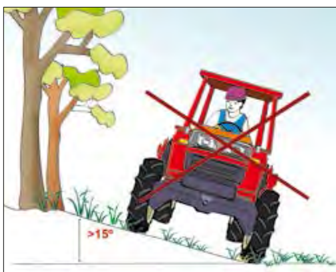
Figure 47c. Avoid operating an agricultural vehicle along a slope exceeding 15 degrees, or use specially designed vehicles and strictly follow the safety rules in using them.
