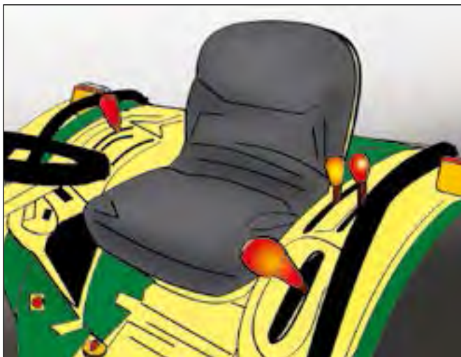
Figure 48c. Control positions and seat arrangements can contribute to good visibility of the surroundings.
