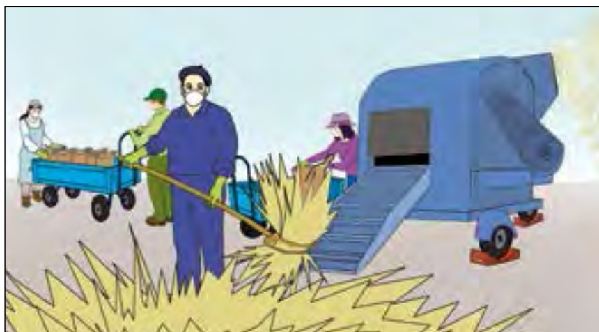
Figure 32a. Use wedges to fix machines with wheels, or use machines with caterpillar tracks.
