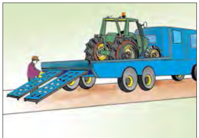
Figure 2f. Use ramps to load an agricultural vehicle onto a truck.
