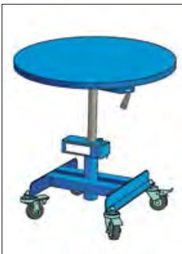
Figure 24c. Design a rotating work-stand at an appropriate height to minimize the lifting of heavy objects.
