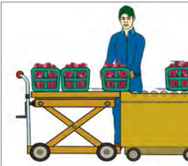
Figure 13b. Minimize height differences between the lift truck surface and the work table.
