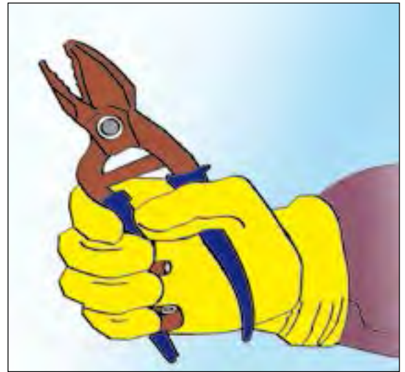
Figure 25b. The grips of tools should have the correct shape and adequate friction.
