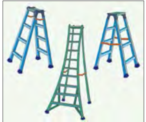
Figure 28b. Stepladders of different shapes are available. Use ladders with arrangements for avoiding sudden collapse.
