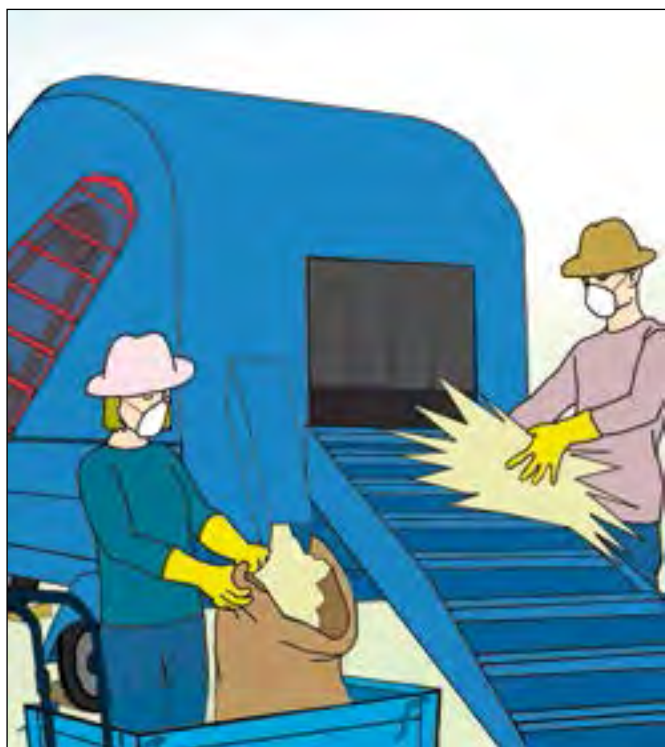
Figure 31a. Feeding device in the form of a conveyor which carries bundles of rice into the dangerous part of a threshing machine.
