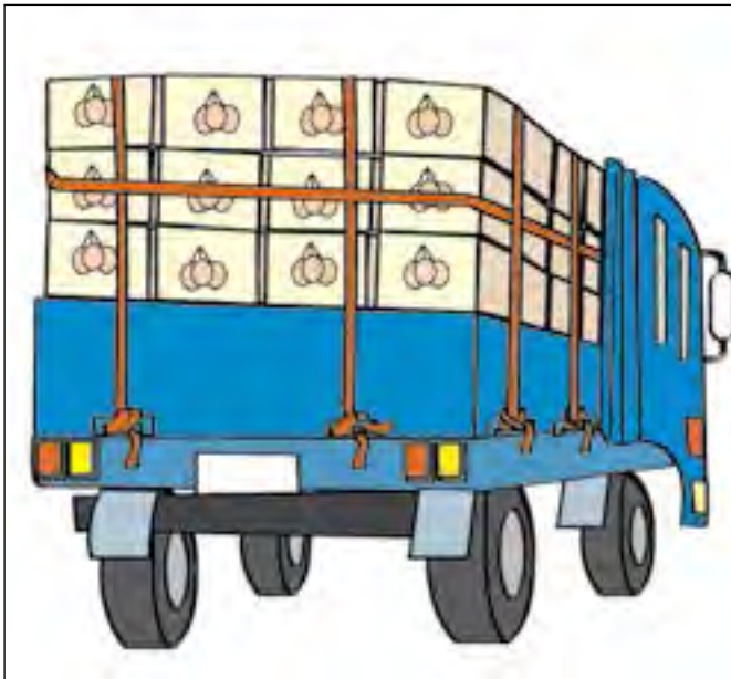
Figure 46a. Put agricultural products in appropriate containers, pile them neatly on the vehicle platform and tie them properly.
