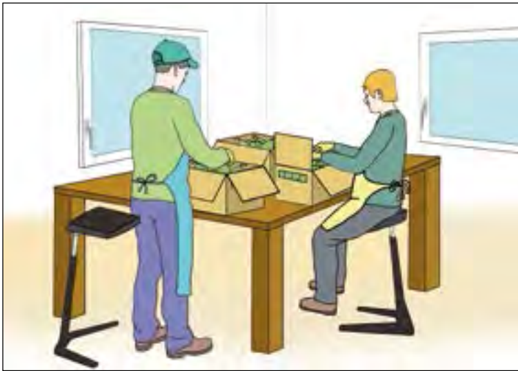
Figure 22a. Provide a chair or stool near the work area; from a standing posture, farmers can occasionally sit on the stool simply by leaning.
