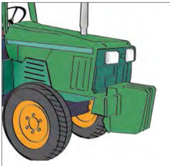
Figure 47a. Add heavy attachments at low positions on a vehicle to lower its centre of gravity.
