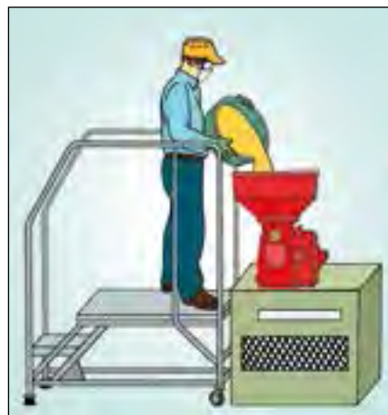
Figure 17d. Adjust the work height by using a stable foot platform corresponding to your elbow level.
