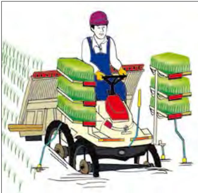
Figure 48a. Ensure visibility from the driver's seat. Good visibility is one of the features of this compact rice-transplanting machine that make it easy to operate.
