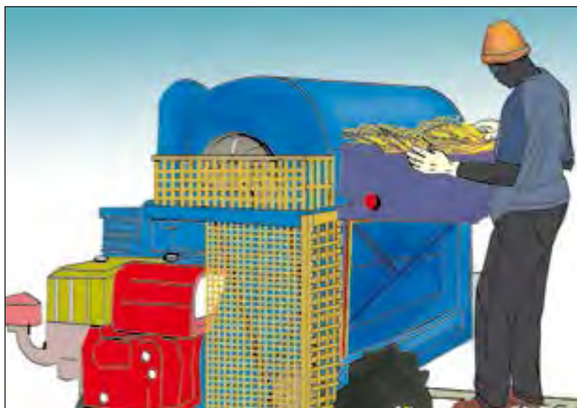
Figure 40a. Make the emergency control of the machine clearly visible, and place it within easy reach of the user.
