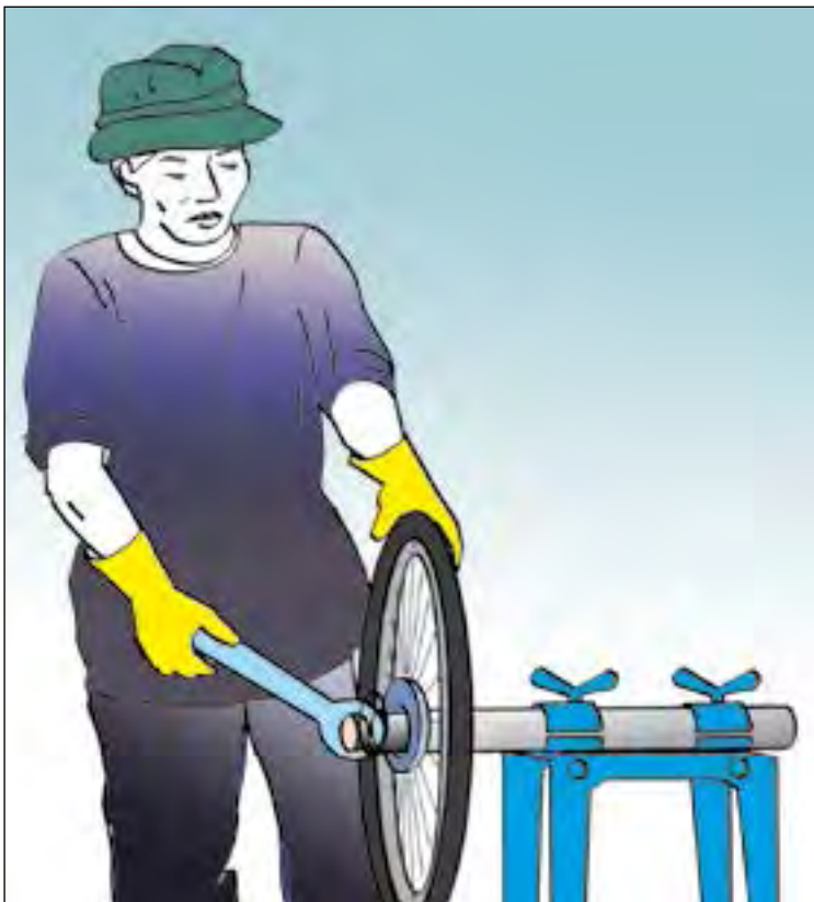
Figure 19c. Use a fixture to hold wheel hubs or axles when they are detached for repair or maintenance.
