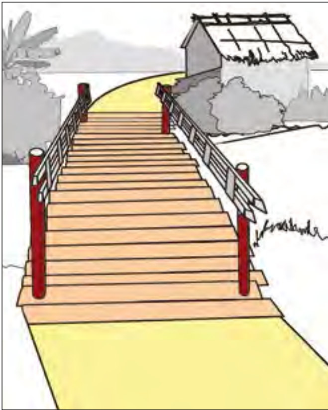
Figure 3a. A bridge, with firm handholds, constructed over a river. The bridge deck is wide enough for the transport of people and farm products.
