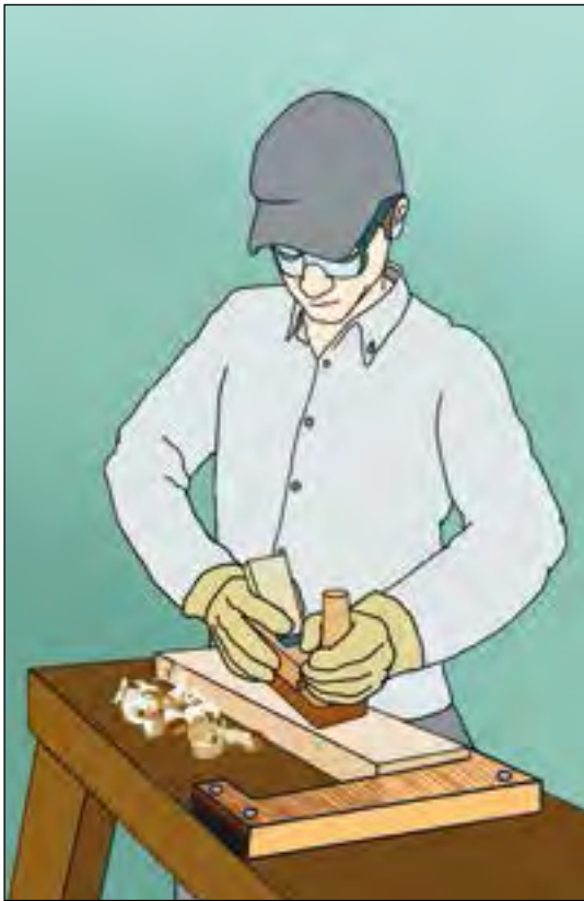
Figure 19a. A low-cost fixture, made of wood, to hold workpieces for planing.
