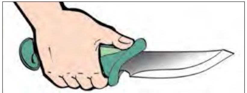
Figure 25c. Sharp tools might injure the fingers if the hand slips. Make sure that such tools are designed properly.
