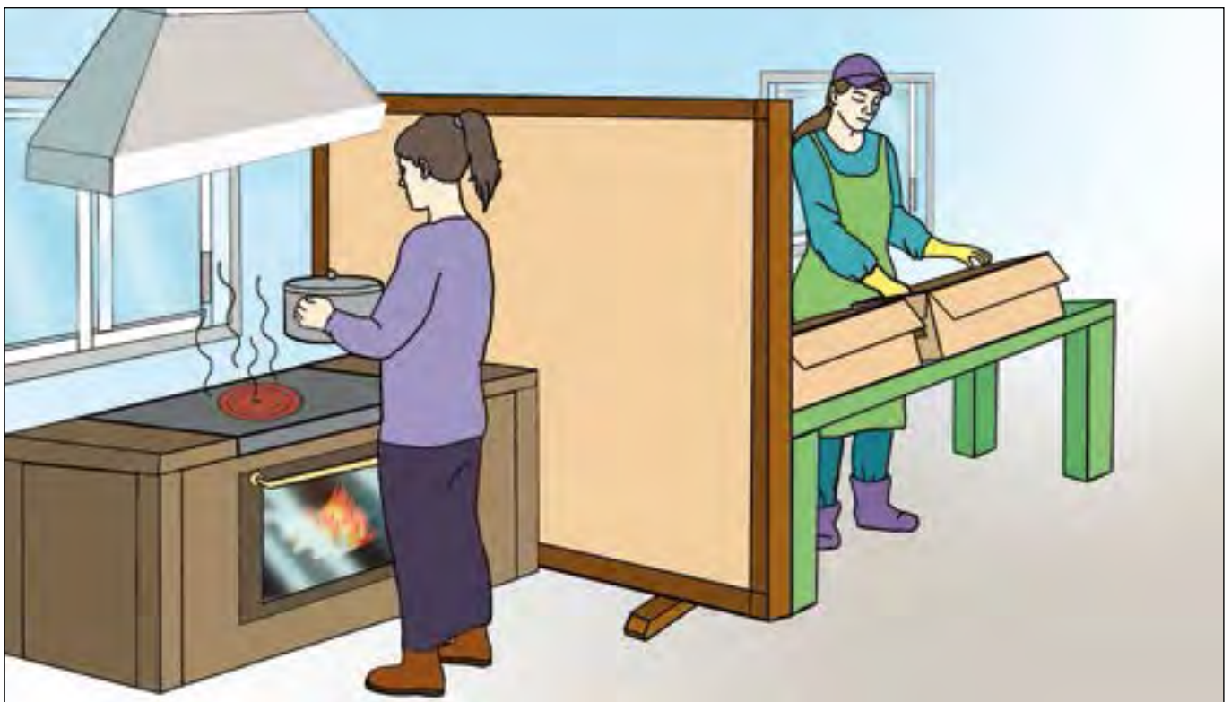
Figure 51b. Make use of screens or barriers to protect workers from heat radiation from heated equipment or walls.
