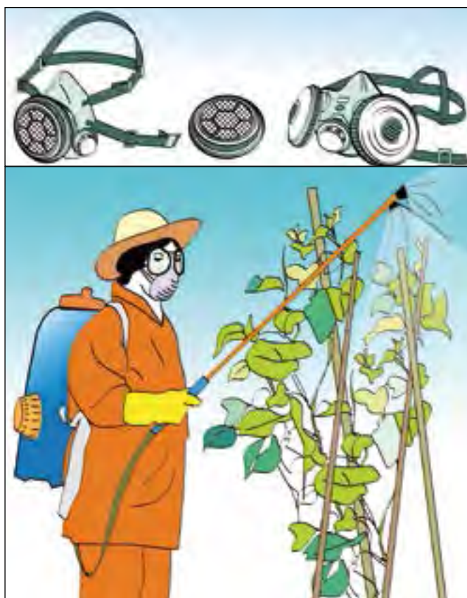
Figure 65c. Mask, with filter containing granules of activated carbon, for use when spraying with pesticides.
