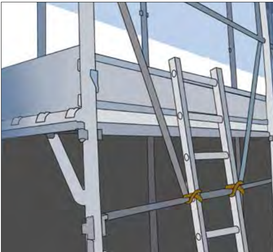
Figure 28c. Ladders for reaching an elevated platform should be securely fastened.
