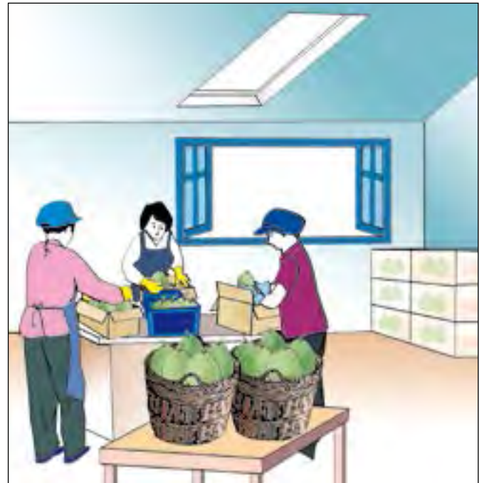
Figure 49b. Use transparent materials or a translucent plastic panel in the ceiling or roof to permit more daylight.
