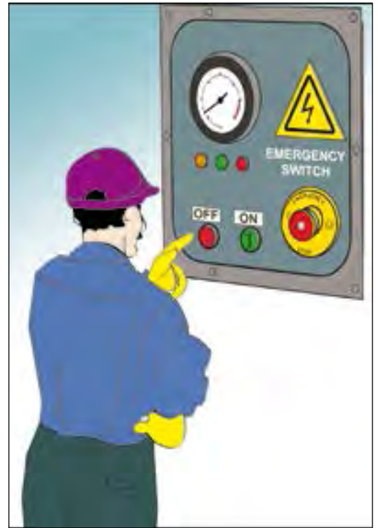
Figure 86b. Use larger letters for labelling switches and displays so that elderly workers can read them easily.
