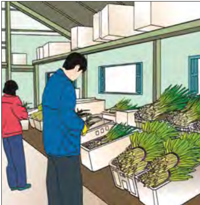
Figure 49a. Choose light-coloured paints (or materials such as white fertilizer bags) to brighten up walls and ceilings. Move the workstation nearer the windows.
