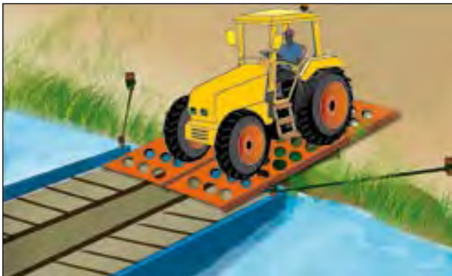
Figure 44c. Provide stable platforms to form a route for vehicles to get on and off a boat.
