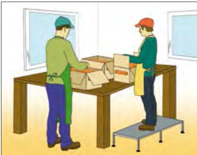
Figure 17b. Use a foot platform for short farmers if the workstation needs to be used by many farmers together.
