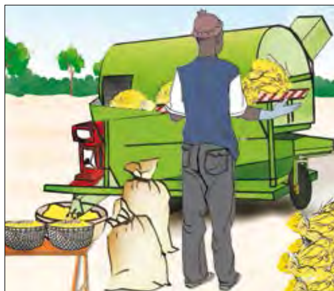
Figure 31b. The feeding part of the machine can be made higher, so that the work is done in a natural standing posture.
