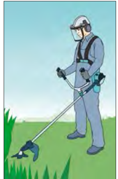
Figure 24b. Use a hand-reaping machine to reduce the workload on your arm and hand muscles. Attach sturdy handgrips to the tool to secure a safe grip.
