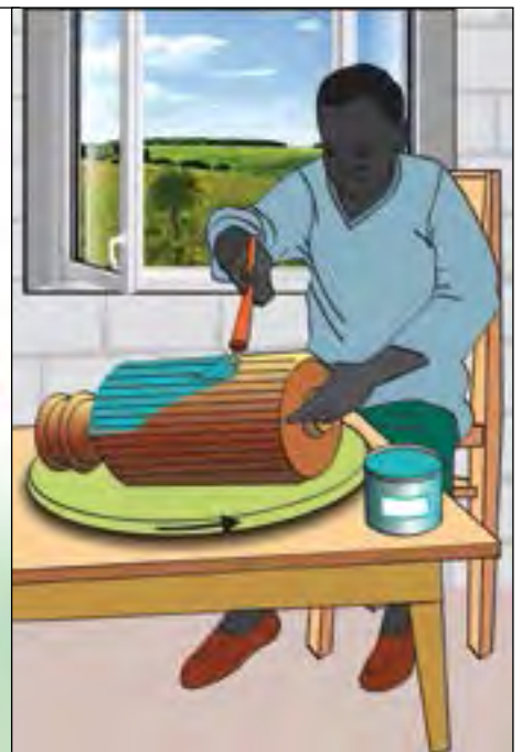
Figure 24c. Design a rotating work-stand at an appropriate height to minimize the lifting of heavy objects.
