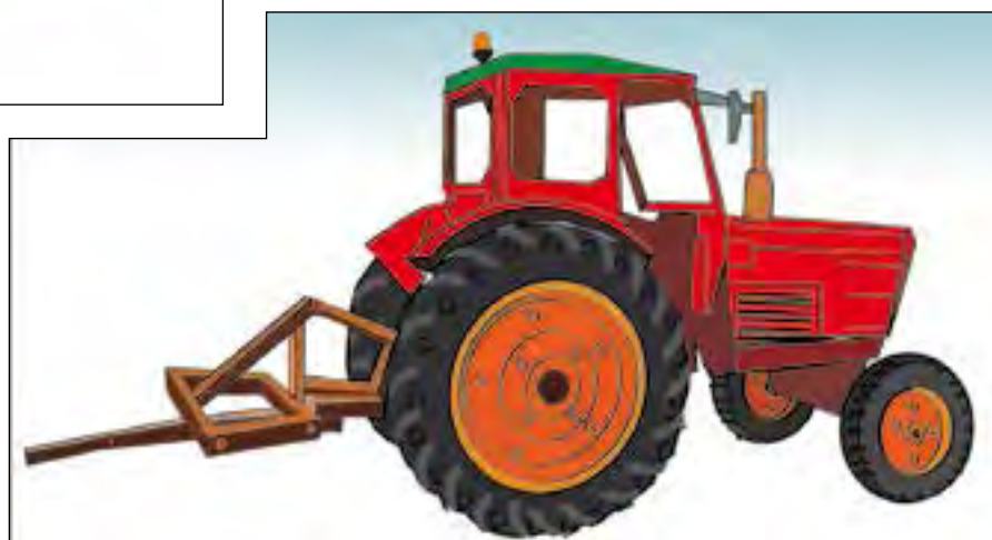
Figure 47b. Attachments at the rear of a vehicle can lower the centre of gravity and act to reduce the risk of unexpected overturning.
