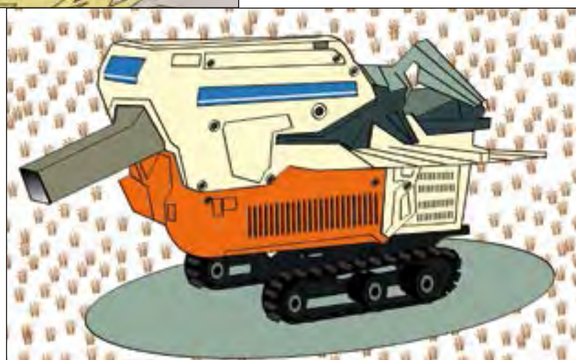
Figure 32a. Use wedges to fix machines with wheels, or use machines with caterpillar tracks.
