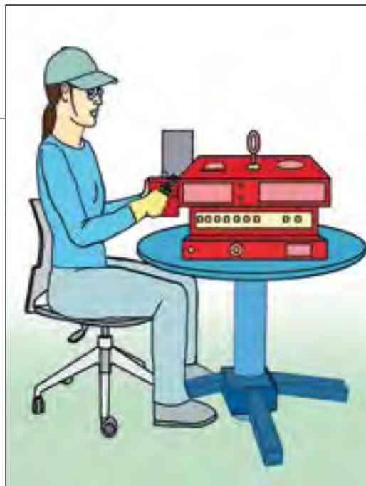
Figure 24c. Design a rotating work-stand at an appropriate height to minimize the lifting of heavy objects.
