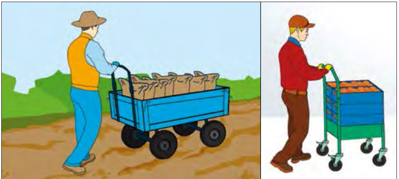
Figure 5a. On rough roads, it is easier to push or pull hand-trucks with large wheels than those with small wheels.
