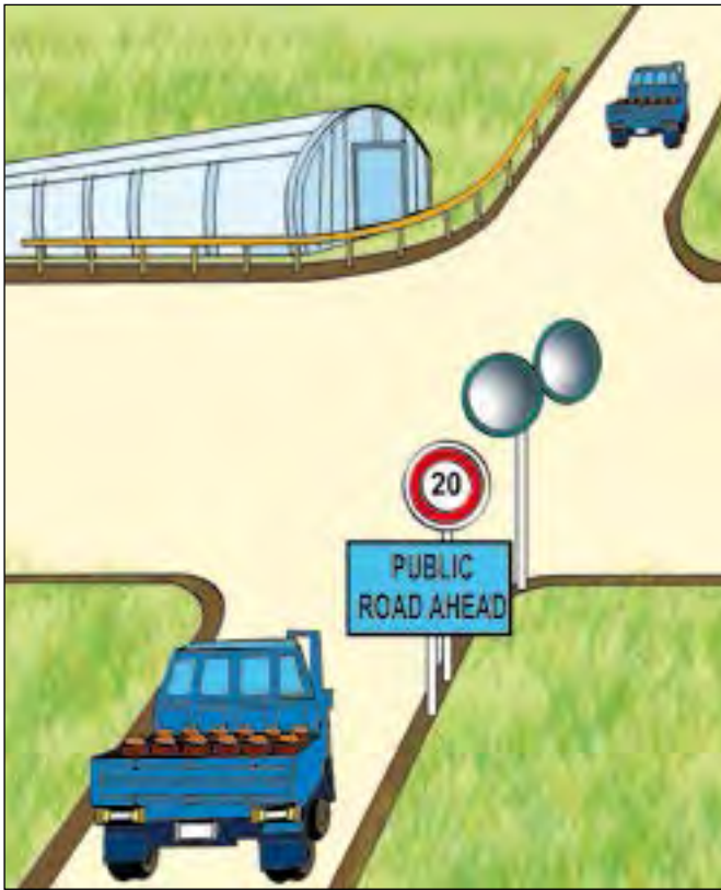
Figure 42a. Put up warning signs and mirrors to ensure safe traffic at junctions with public roads.
