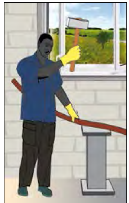
Figure 17e. When greater force is needed for work, choose a work height slightly lower than your elbow height.
