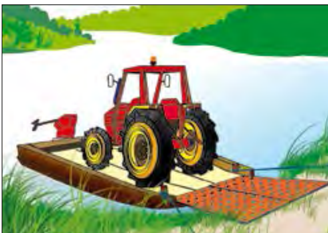
Figure 2e. Use a ramp to load a vehicle onto a boat safely.
