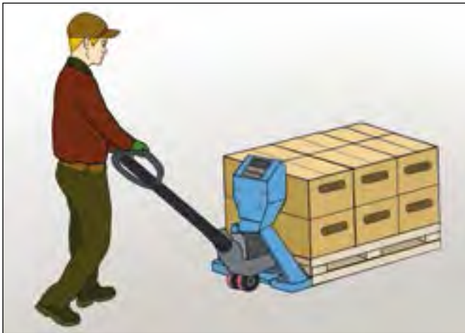
Figure 11a. A manually powered device to move pallets with heavy items.
