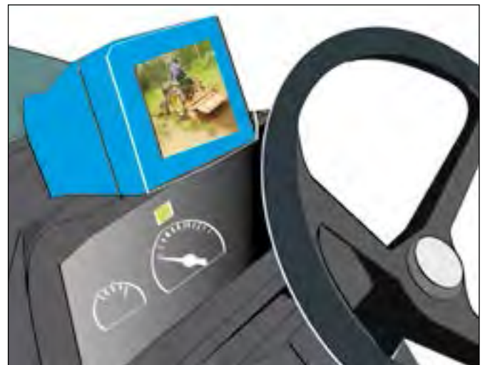
Figure 48d. Visibility from the driving seat can be improved by a special screen showing the image from a camera on the front or rear of the vehicle.
