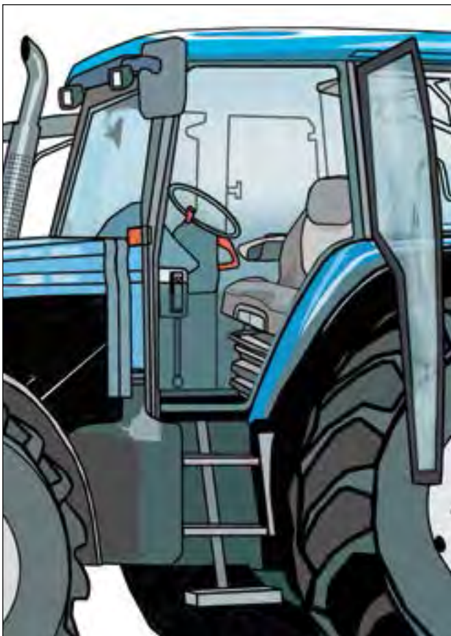
Figure 45b. Easy access to the driving seat, proper seating and measures to protect from weather conditions and to reduce noise and vibration are important to prevent slippages, maximize seating comfort and avoid mistakes in operation.
