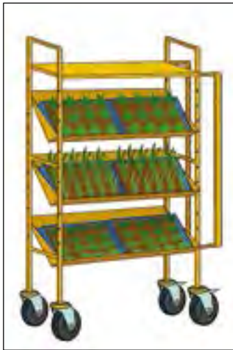
Figure 10a. Mobile racks can reduce the number of trips.
