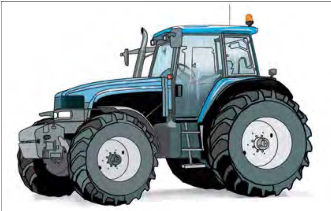
Figure 45a. All tractors should have in place a Roll-over Protection Structure (ROPS) which combined with a safety belt will avoid most of the fatal accidents.
