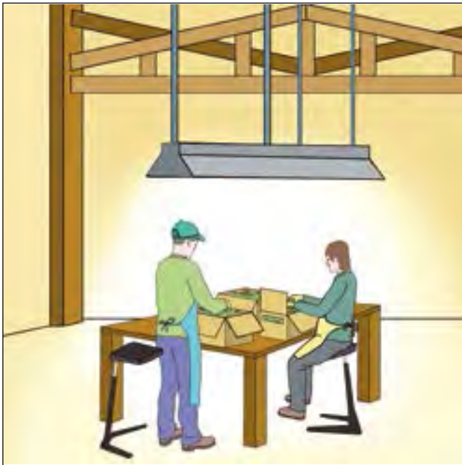
Figure 50a. Relocate lights to obtain sufficient lighting for precision or inspection work.
