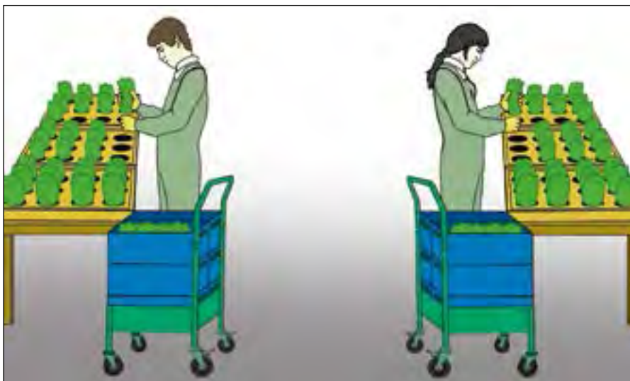
Figure 18b. Arrange work tables and trolleys so that work is done without bending or twisting of the body.
