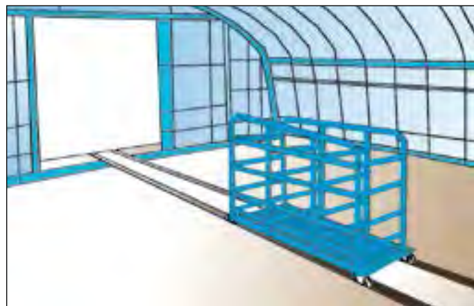
Figure 10g. Multi-level shelves can also be mobile along a route.
