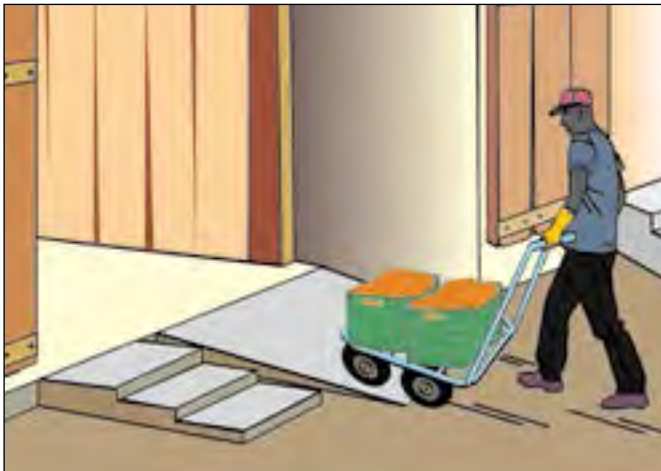
Figure 2a. Provide ramps with a small incline over the sudden height difference at the entrance to a building.
