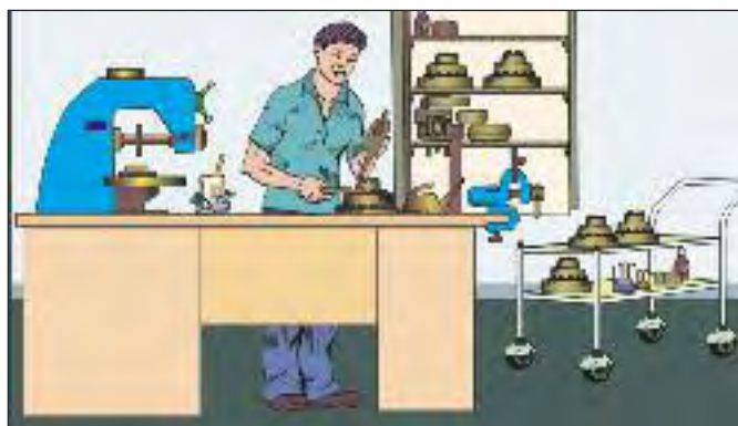
Figure 118a. Provide multitask workstations for use by different workers. This helps the enterprise organize a better flow of work.
