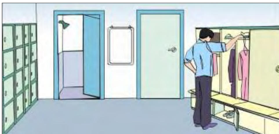
Figure 95a. Arrange for gender-separated changing rooms with lockers and clothes racks allocated to individual workers.
