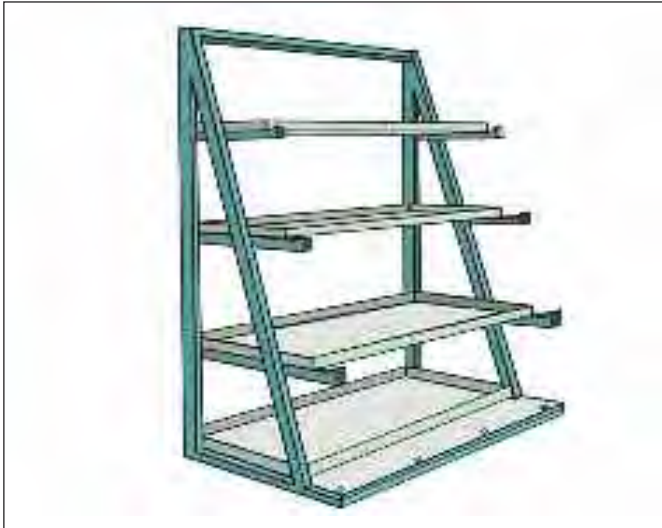
A vertical rack. Tray-type shelves provide room for small pieces.
