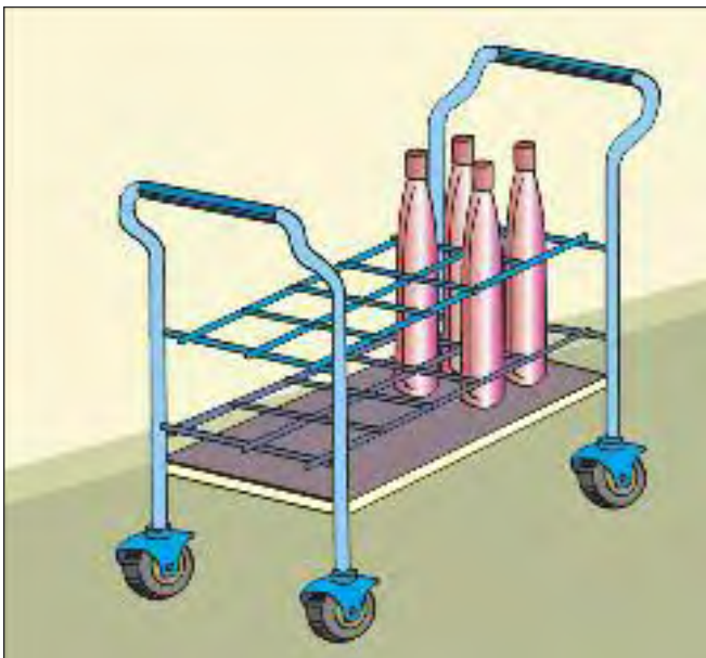
Figure 7c. A rack on wheels specially designed for storage and handling of motorcycle silencers.
