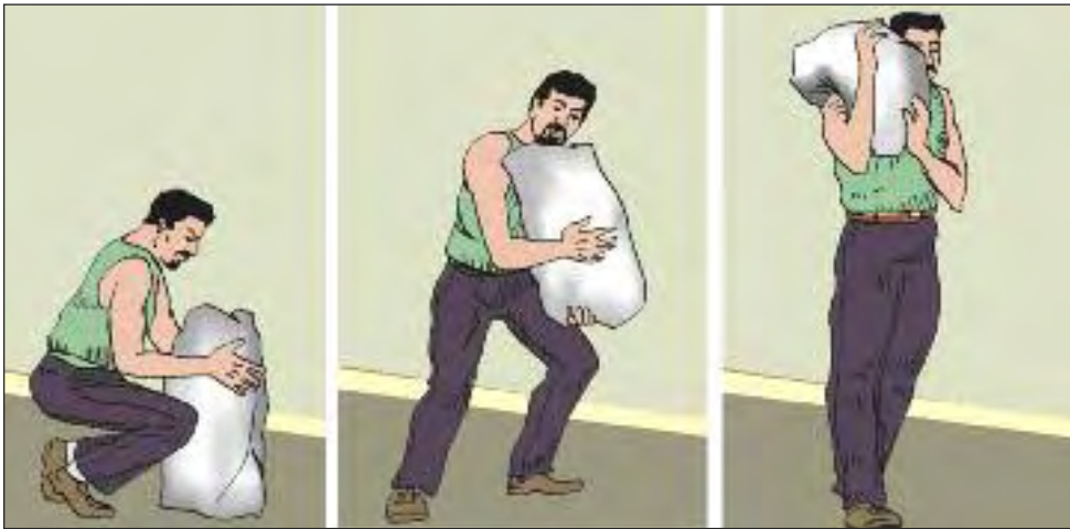
Figure 15a. Do manual lifting or lowering of a heavy load in front of the body, with the back kept straight and with stable feet positions, and use the power of the legs.
