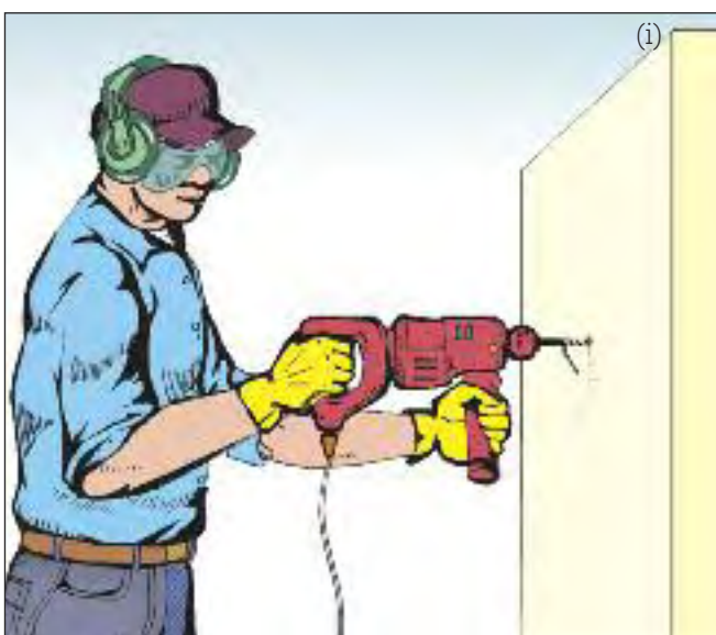
Figure 18c. (i) and (ii) Steady grips of power tools help reduce the required force of operation.
