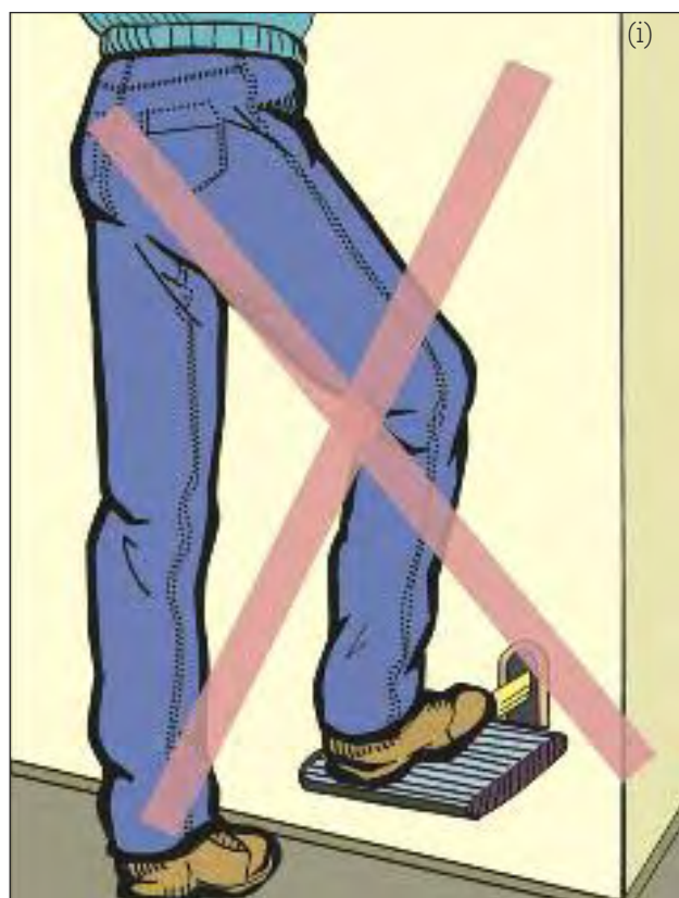
Figure 38b. (i) A pedal level that can be reached only by raising the foot away from the floor is tiring. (ii) Make the pedal level lower and provide a foot platform for easy pedal operation.
