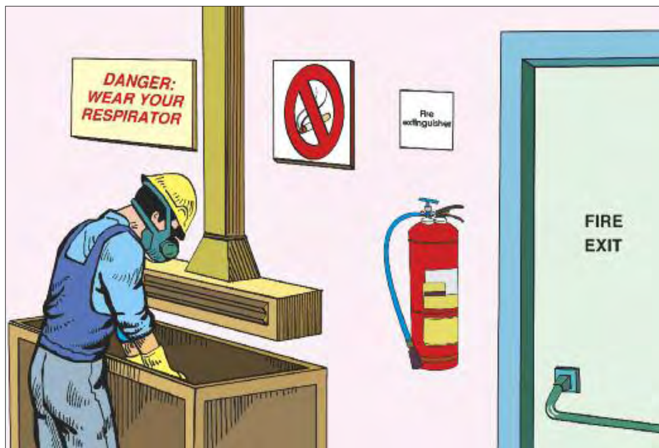
Figure 100. Clearly mark areas where the use of particular personal protective equipment is obligatory.
