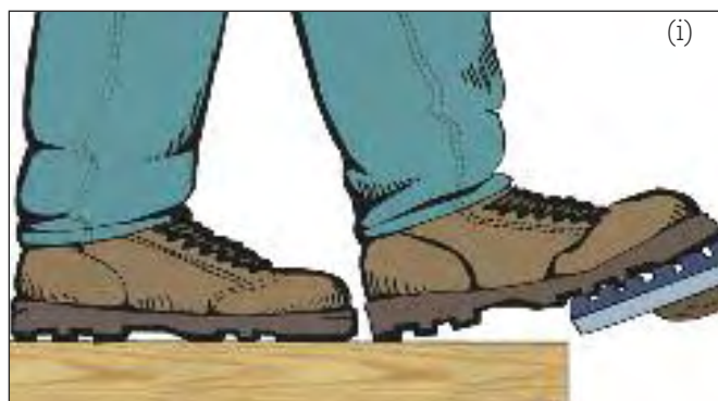
Figure 38a. (i) and (ii) Locate a foot pedal at floor level and make the pedal large enough for easy operation.
