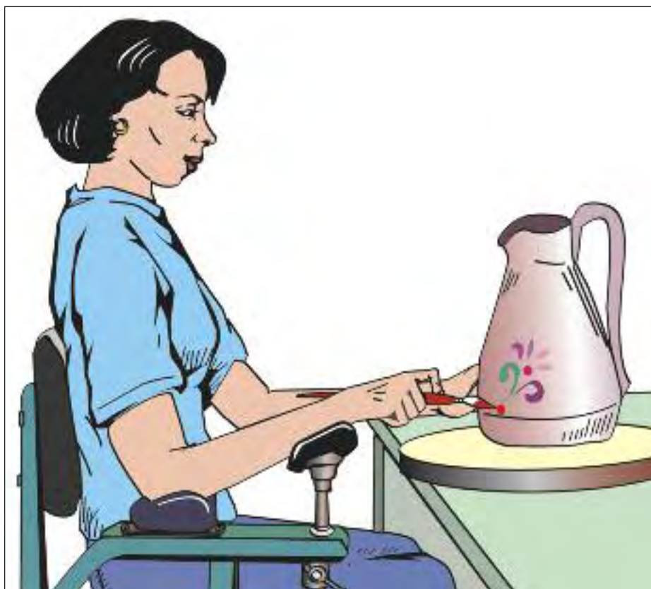
Figure 22a. A hand or forearm support near the point of operation increases the efficiency of precision work.
