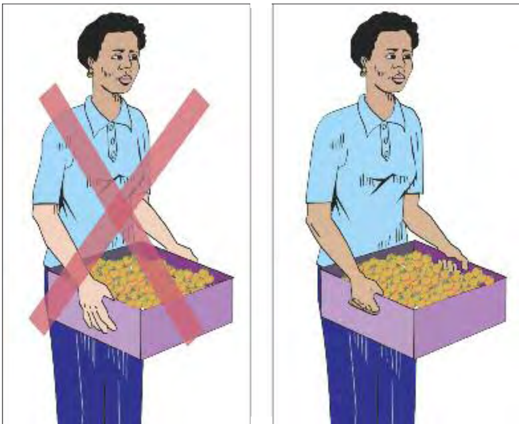
Figure 12b. Cut-out handholds are very useful. Locate these handholds so that the box or container can be carried in front of the body.
