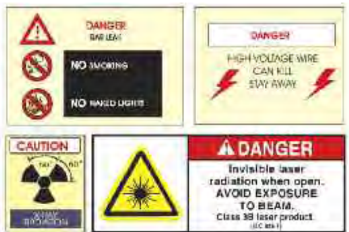
Warning signs should use short messages that indicate the nature and gravity of the hazards.
