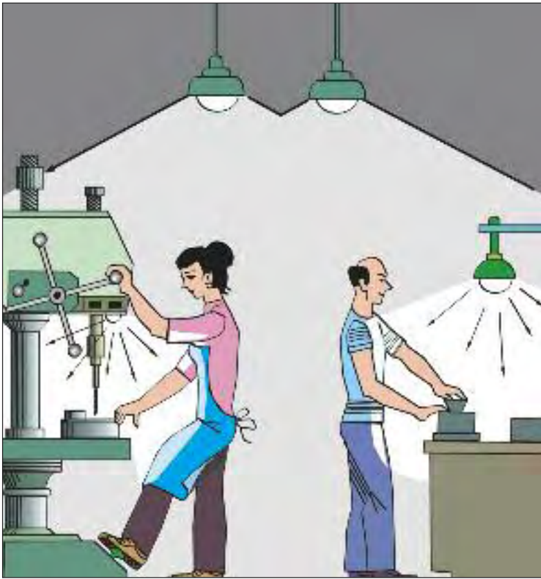
Figure 69a. A combination of general and local lights helps to meet the specific requirements of different jobs.
