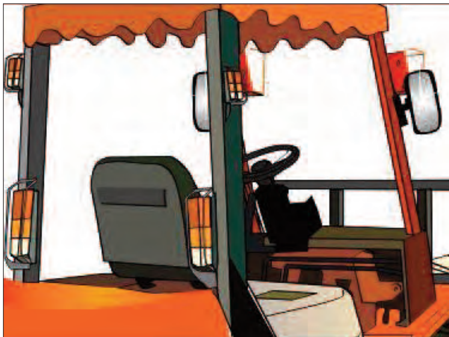
Figure 63b. Provide mirrors and lights at appropriate positions to allow wide visibility in various operating situations.
