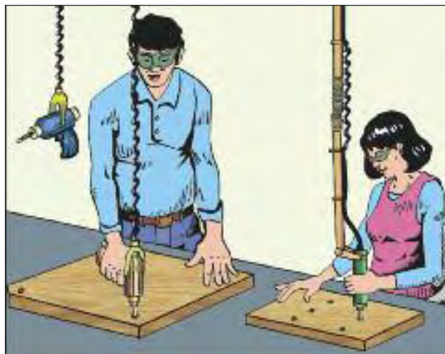
Figure 20b. Hanging tools within easy reach of workers are suited to repeated operations.
