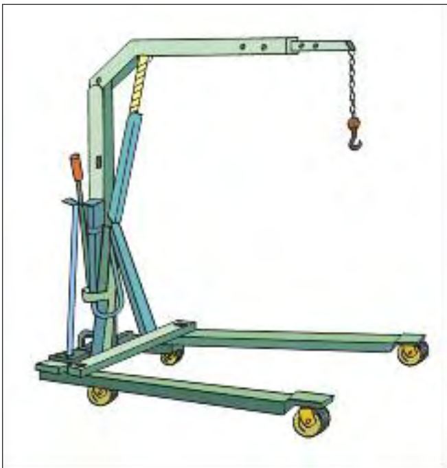
Figure 9c. A manually powered hydraulic floor crane with a telescopic boom.
