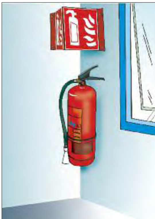
Figure 81a. Provide sufficient fire extinguishers at clearly designated places within work areas.
