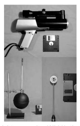
**FIGURE 60.5** Three types of radiation measurements: bottom left: black globe with mercury thermometer in center; bottom right: unidirectional sensor, using the temperature measurement of a reflective and an absorbing surface to calculate radiation levels; top: infrared radiation meter, a spot-meter with a small measuring angle, hence the visor to aim precisely at the correct spot.
