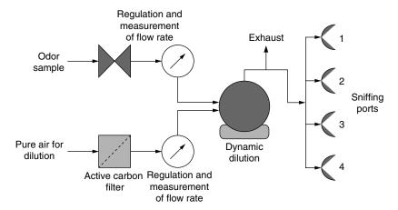
FIGURE 66.1 Schematic representation of an air dilution olfactometer.
