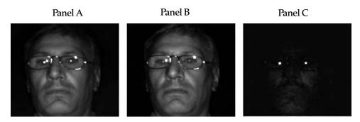
**FIGURE 25.1** The three images obtained by PERCLOS are shown. The "bright-eye" image (Panel A) and the "dark-eye" image (Panel B) are essentially identical except for the glowing pupils in the "bright-eye" image. The difference image (Panel C) eliminates all image features except for the bright pupils.
