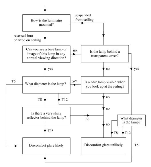
**FIGURE 69.1** A flow chart for identifying fluorescent lamp/luminaire combinations likely to produce discomfort glare. The answers are given by an observer sitting at a workstation. For identification purposes, the diameters of the three most common fluorescent lamp types are T12 = 38 mm (1.5 in.); T8 = 25 mm (1.0 in.); T5 = 16 mm (0.63 in.).
