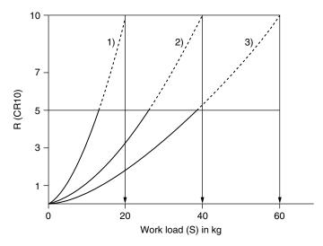
**FIGURE 11.2** The figure shows the form of S–R functions for muscular effort and how functional capacity can be extrapolated from submaximal responses.
