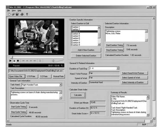
FIGURE 9.1 Calculations of strain index for chair-drilling task.
