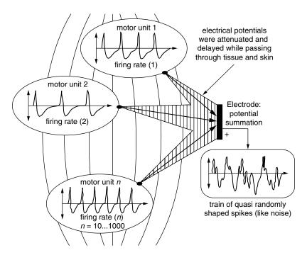
FIGURE 19.1 EMG signal composition using surface electrodes.
