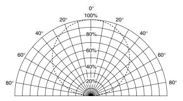
**FIGURE 68.8** Cosine response of a high-quality illuminance meter. This figure shows that light incident on the illuminance meter at, for example, 50° will be approximately 65% as effective as the same light intensity at 0°. (Image courtesy of the Lighting Research Center, Rensselaer Polytechnic Institute.)
