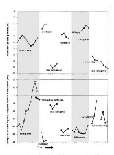
**FIGURE 20.1** Average heart rate (top panel) and the 0.10-Hz component of HRV (lower panel) during test rides in a driving simulator (N = 22). Time is displayed in steps of 10 sec. HRV is displayed compared with a resting level of 0. (Adapted from De Waard, D. [1996], The Measurement of Drivers' Mental Workload, Ph.D. thesis, University of Groningen, Groningen, the Netherlands. With permission.)
