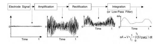
FIGURE 19.2 Recovering the intensity function from a surface EMG.
