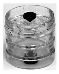
FIGURE 64.7 Filter cassette for collecting dust samples.
