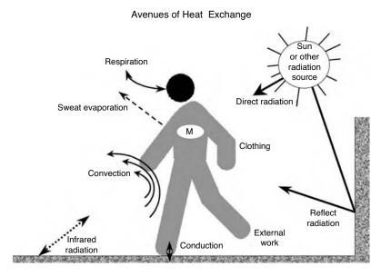
**FIGURE 60.2** Schematic representation of the pathways for heat loss from the body. M = metabolic heat production. (Reproduced with permission from Havenith, G. [1999], *Ann. Occup. Hyg.*, 43, 289–296.)
