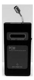
FIGURE 64.4 Direct-reading particle counter.
