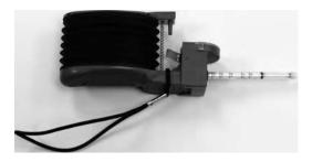
FIGURE 64.2 Handheld pump and gas detector tube.
