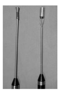
**FIGURE 60.3** Example of shielded (radiation) ambient temperature sensor (right) and contact temperature sensor (left). This shielded sensor cannot be used with very high radiation levels because the single shield is in close proximity to the actual sensor, and without ventilation of the space in the shield, the shield would heat up and affect the sensor through radiation.
