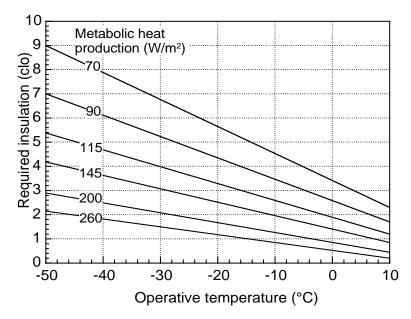
**FIGURE 61.1** Neutral IREQ as a function of ambient operative temperature at six levels of metabolic heat production. (Modified from ISO TR 11079 [1993], Ergonomics of the Thermal Environment: Cold Environments, Determination of Required Clothing Insulation [IREQ], International Organization for Standardization, Geneva.)
