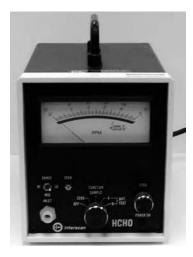
FIGURE 64.3 Direct-reading formaldehyde meter.
