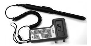
FIGURE 64.5 Multichannel IAQ monitor and data logger.
