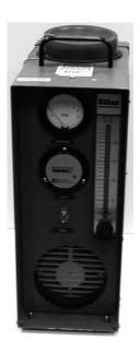
FIGURE 64.8 High-volume sample pump.
