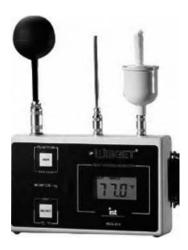
FIGURE 62.1 Heat stress monitors.
