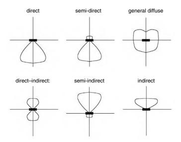
**FIGURE 68.2** Luminous intensity distributions for different types of light fixtures. Every black rectangle represents a light fixture centered along vertical and horizontal axes. The solid lines represent the luminous intensity distribution emitted from the different types of fixtures. All but the "direct" fixture would be mounted below the ceiling plane. (Image courtesy of the Lighting Research Center, Rensselaer Polytechnic Institute.)
