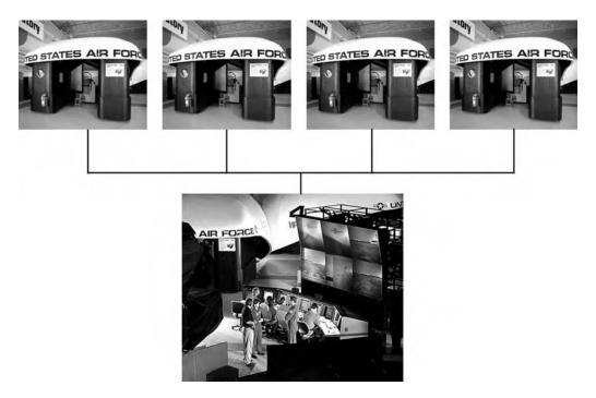
**FIGURE 45.1** Air force distributed mission training center. Four fighter cockpits inside wraparound 360-degree visual domes. An instructor/operator station outside of the four networked simulator domes.
