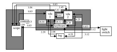
FIGURE 28.1 Link analysis of electron-microscopy workstation.
