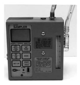
FIGURE 64.6 Low-volume programmable sample pump.
