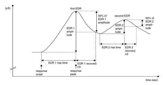
**FIGURE 18.3** A typical electrodermal response (EDR) with its parameters (rise time, amplitude, recovery time) as measured by the application of an external voltage. Recovery t/2 refers to falling back to half of the amplitude. In the event that a second EDR starts prior to reaching this point, which is not the case in the example shown, EDR recovery t/2 can not be obtained without extrapolation.
