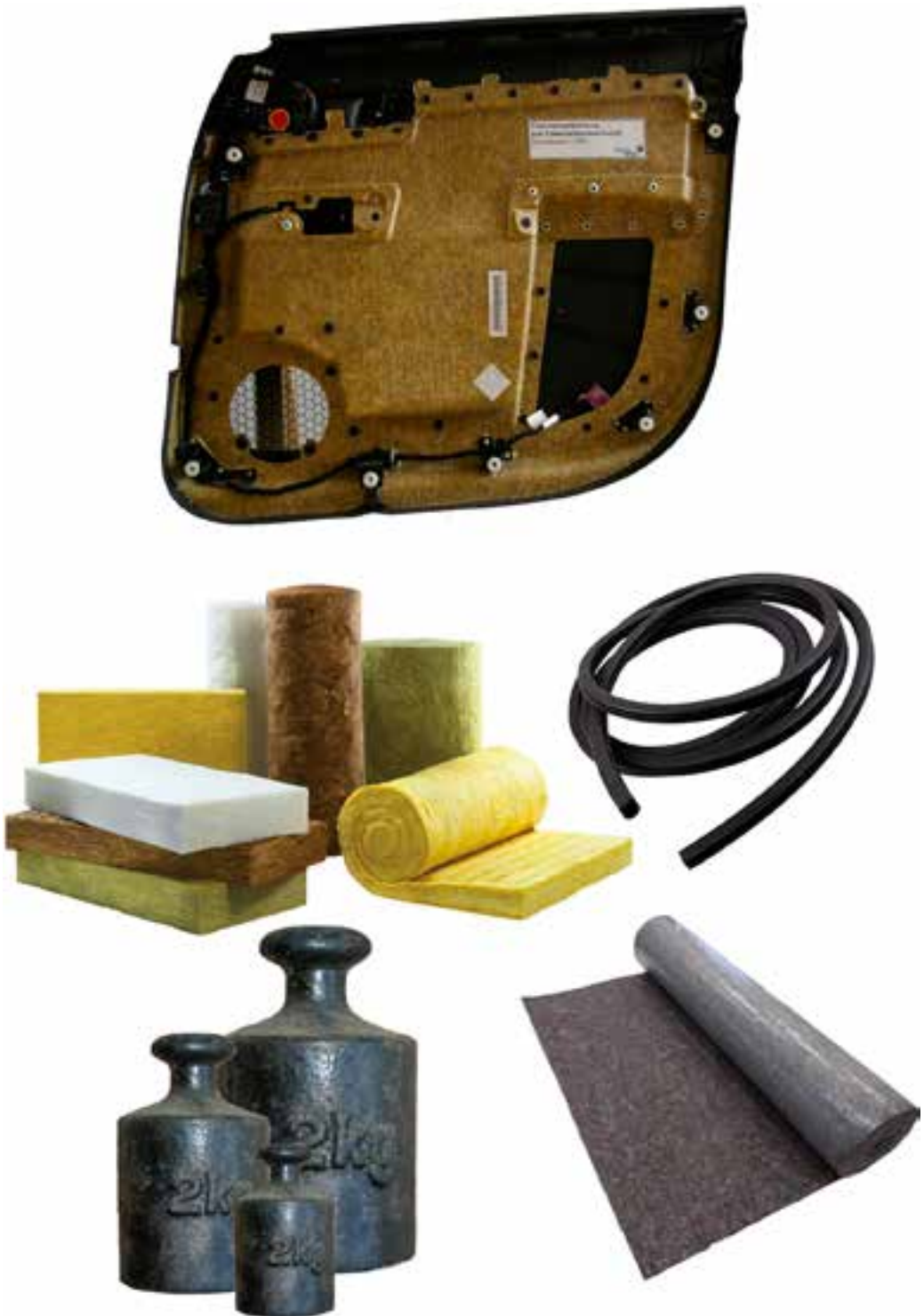
FIGURE 7.5 Designing sound at times means stuffing material into a car door. The pricier your car the more silent it is inside, the more solid are the built-ins (Bijsterveld et al. 2014).
