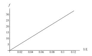
The graph has frequency in Hertz along the vertical axis and 1/L in inverse meters along the horizontal axis. The function found by the least squares fit procedure is f = 276(1/L) + 0.037. We shall assume that this fits either the model of an open organ pipe (mathematically similar to a string fixed at both ends) or that of a pipe closed at one end.
